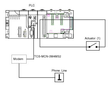
(1): the actuator is connected on the channel 0 of the discrete module.
