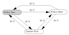
**NOTE:** In order for changes to be made from one protocol to another, the processor must initially be configured to Modbus Slave mode.
