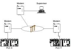
The devices communicate with each other using modems. The supervisor is Modbus master whereas the X and Y PLCs are slaves.
