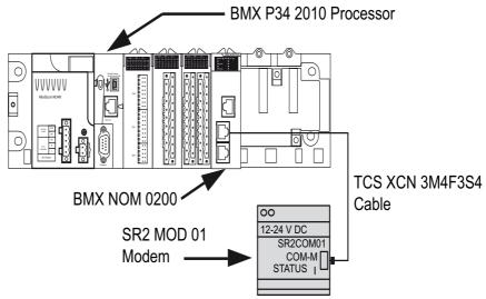
The modem connection needs specific modem cable to work.
