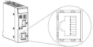
The RJ45 connector has eight pins. The pins used vary according to the physical link used.
