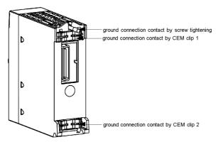
These contacts connect the grounding bus of the modules to the grounding bus of the rack.
